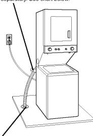
Floor drain system: Requires a siphon break, see chart below. A minimum carryaway capacity of 17 gallons per minute is required.
